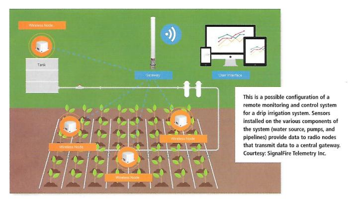
in Modbus format then manages outbound communications by formatting data for delivery to a control center. An Ethernet interface module can tie information from the gateway into a web-based tool such as a laptop or cell phone.
